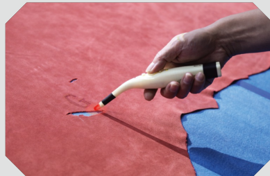
Electric marking defects
